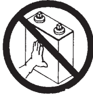
DO NOT PUSH ON CENTER TO POSITION BATTERY
