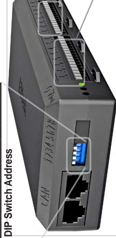
Load Monitor Module
